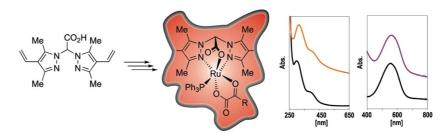
The new scorpionate ligand bis(3,5-dimethyl-4-vinylpyrazol-1-yl)acetic acid (Hbdmvpza) is suitable for copolymerisation with MMA or EGDMA. Immobilised manganese, rhenium, iron and copper
