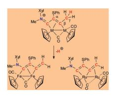
Conjugated iminium ions (as bridging vinyliminium ligands) can undergo  $\gamma$ -deprotonation to form dienamines, which are stabilized by dinuclear coordination. Two different coordination modes have been evidenced.
